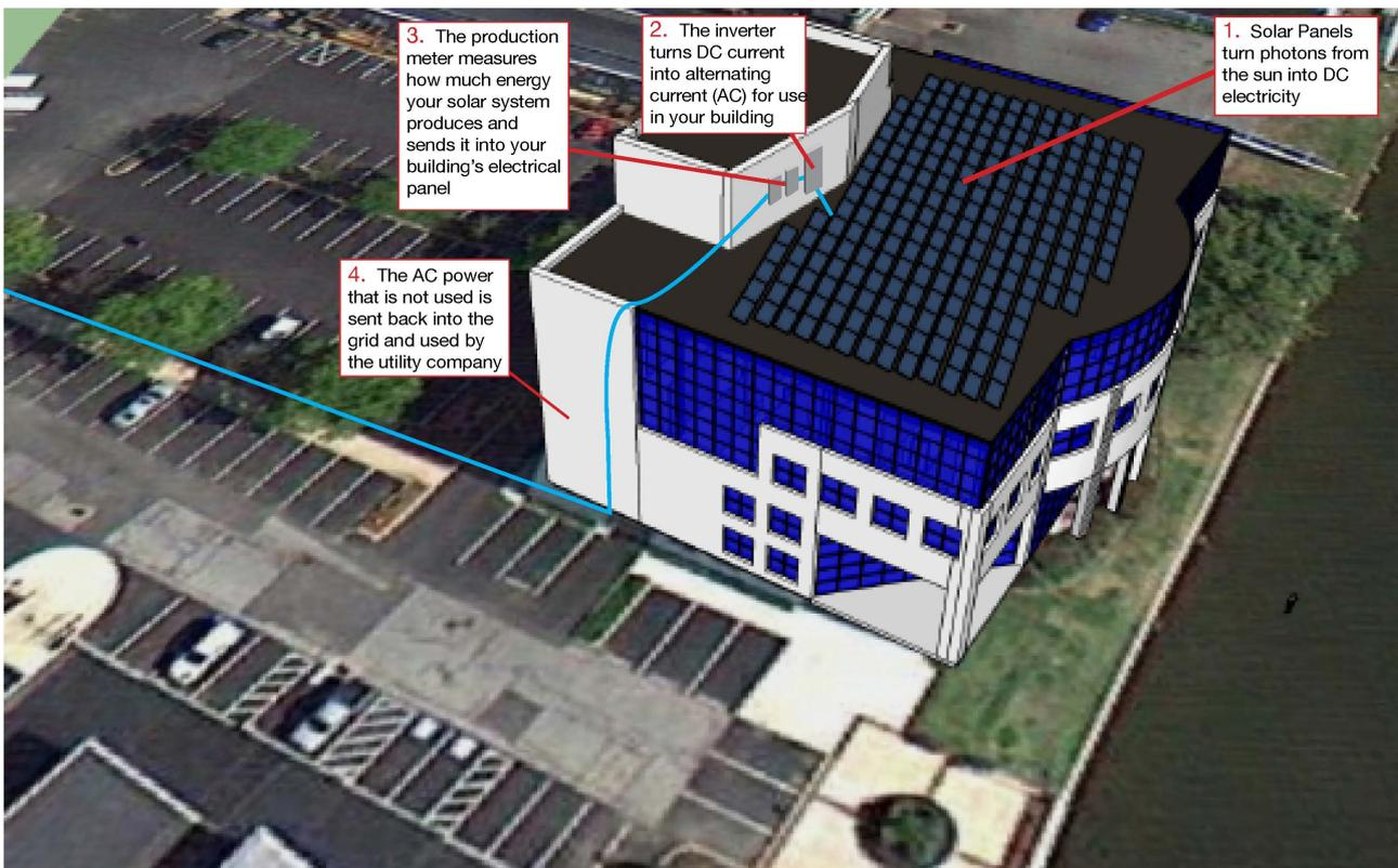
**Solar electric power** begins with the **solar panel**. Each solar panel receives energy from the sun as photons. What is a photon?
